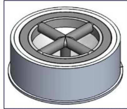
ALCOA Flight Deck Tie Down Assembly 05003554 Substitute For PK-T50 USN Decking LCS Type Ships with Aluminum Deck
