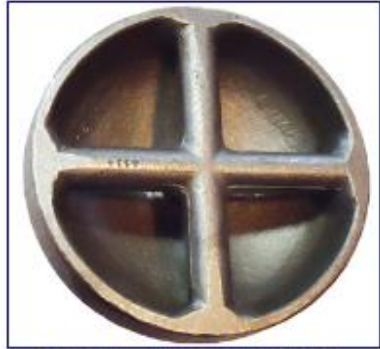
Type 14 - Type XIV US Navy Aircraft Tie Down - Flush For Welding Into Steel Deck Type 14 (Replaces Type 1) Type XIV (Replaces Type I) Per NAVSEA Drawing 803-1916300
