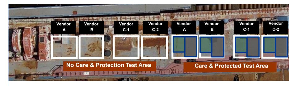
Test areas are set up to determine the most effective and efficient methods to clean ,care and protect nonskid coatings through the build cycle.
