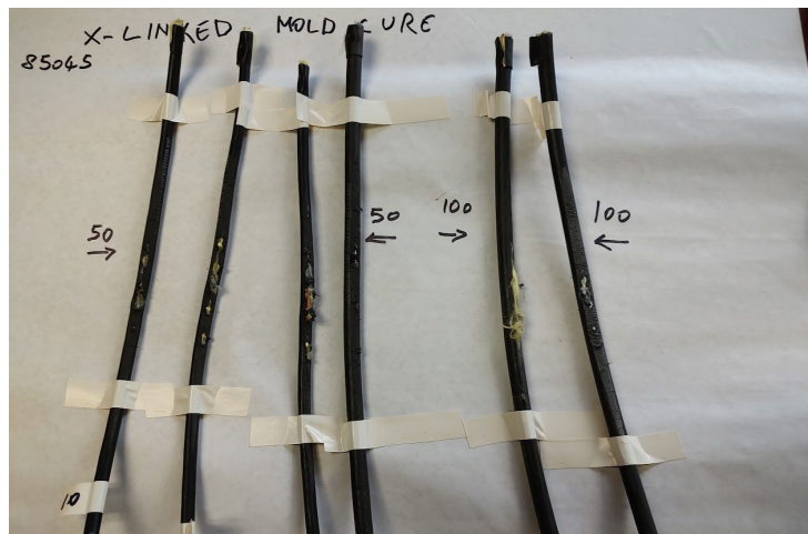
Thermoset Mold Cure X-Link (Fail @ 50 to 100 Cycles)
