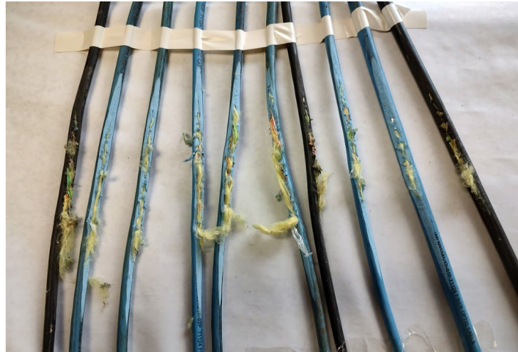
Thermoset Irrad X-Link (Fail @ 50 Cycles)
