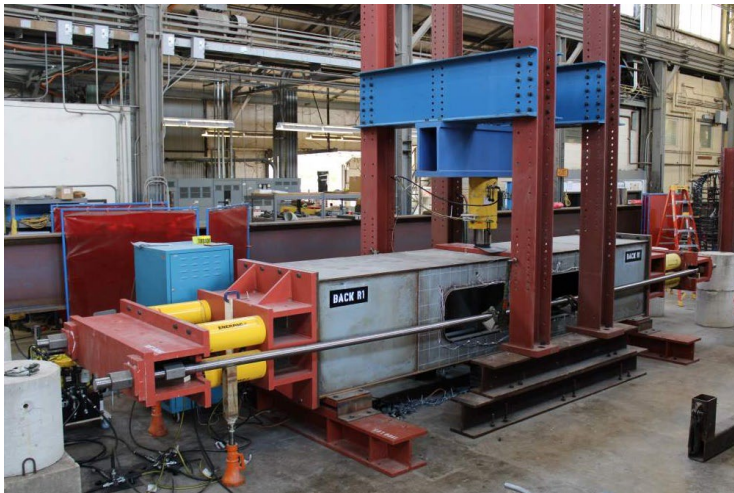
Reinforced Opening Specimen #1 Installed in the Test Fixture
