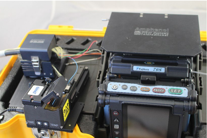
Several inches of splice clearance needed
