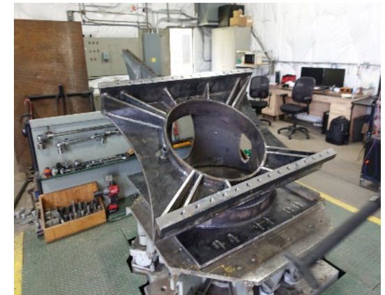
(above) Deck Simulating Shock Machine (DSSM) Test Fixture Design; (below) Universal Medium Weight Fixture Design
