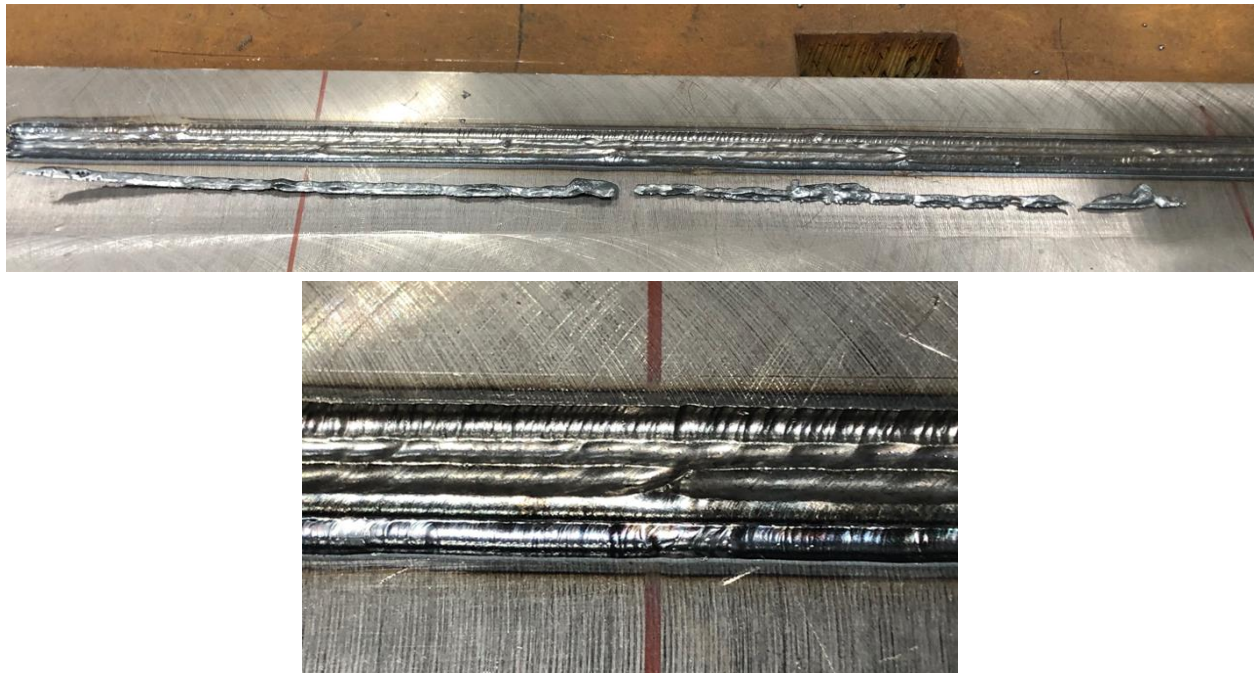
Figure 14. Excavation by Multiple Single-Pass Gouges
