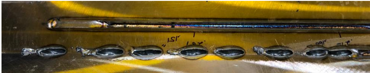
Figure 9. Successful Gouge Followed by Failed Initiation Attempts
