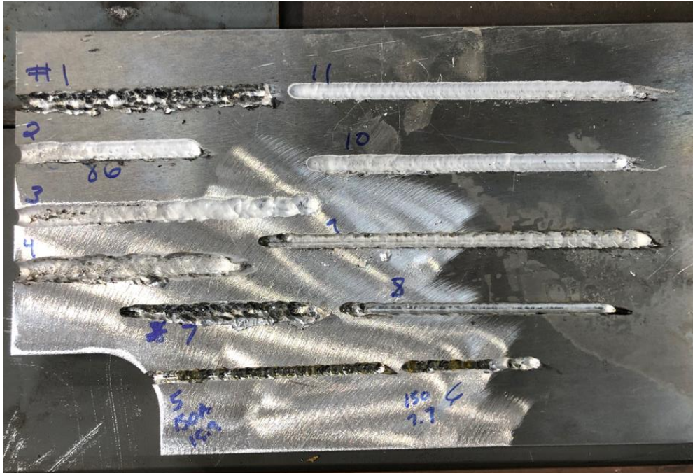
Figure 22. Gouge Trials Made on 5085 Aluminum
