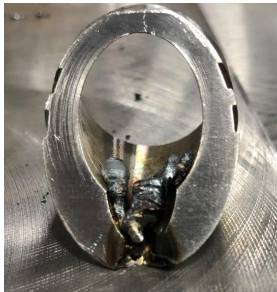
Figure 6. New Tip with Integrated Sip Port (left) and Partially Melted and Clogged Tip after Making a Short Gouge (right)
