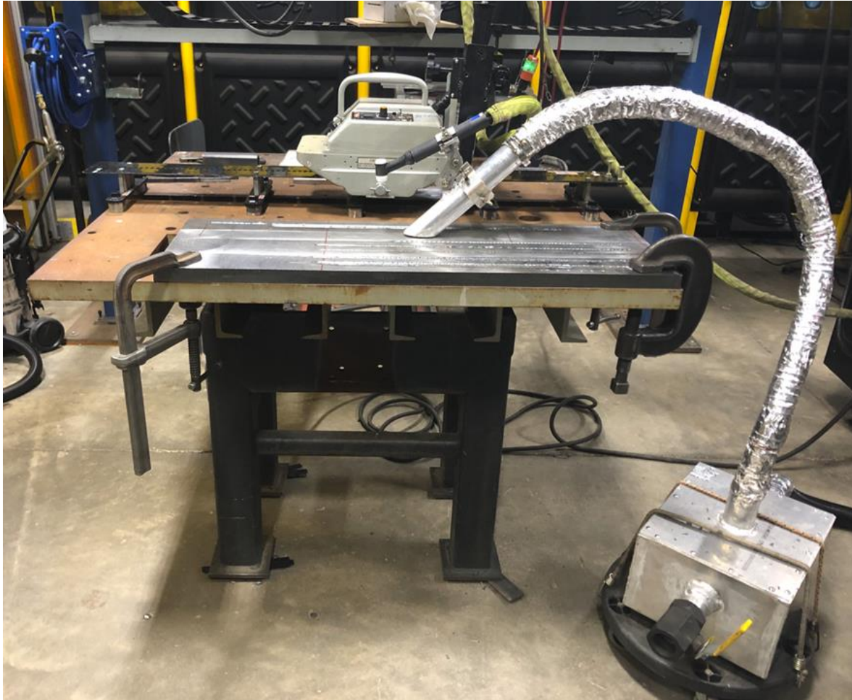
Figure 4. WeldVac Mounted on a Gulco Welding Tractor
