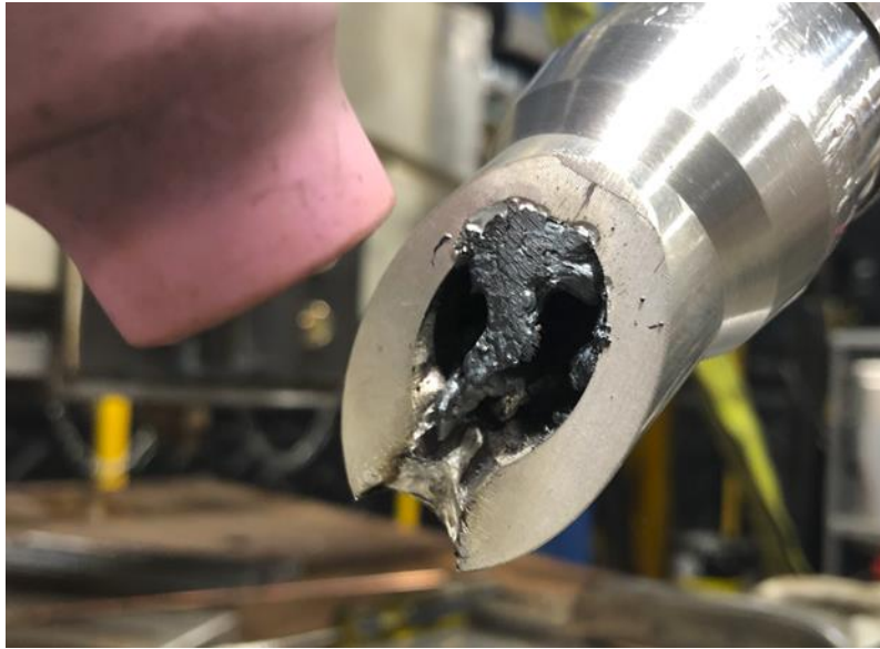
Figure 7. Melted Tip with Significant Geometrical Changes to the Sip Port.
