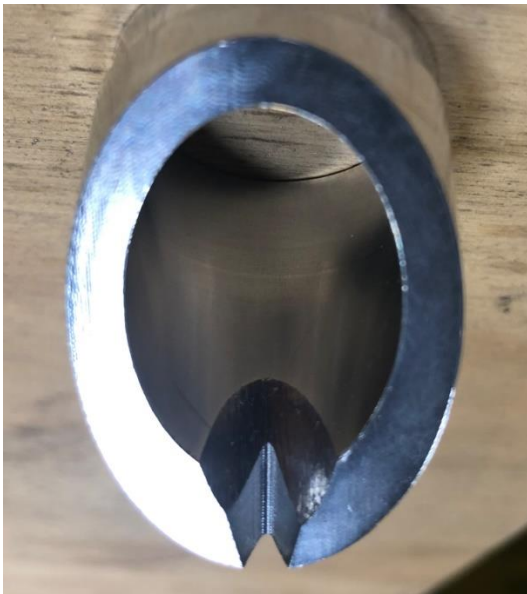
Figure 6. New Tip with Integrated Sip Port (left) and Partially Melted and Clogged Tip after Making a Short Gouge (right)
