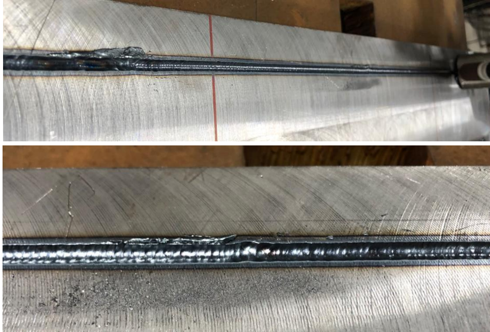
Figure 13. Single Gouge with One-Piece Torch
