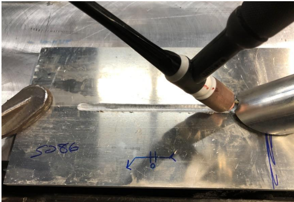
Figure 27. Back-Gouged Trial on 5086 Aluminum Plate
