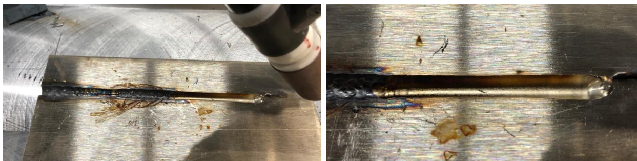
Figure 19. Initial Gouge Trial on 70-30 Cu-Ni
