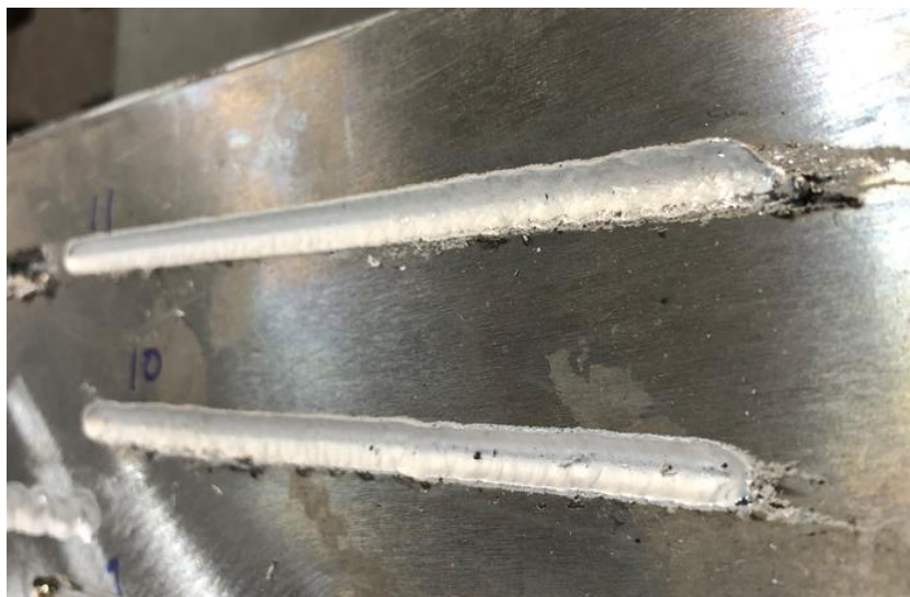
Figure 23. Good Gouges Made with 100% Argon Shielding Gas
