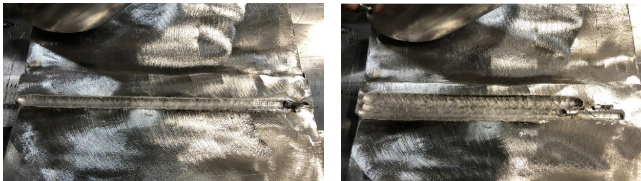
Figure 24. Weld Reinforcement Removal from Aluminum Plate
