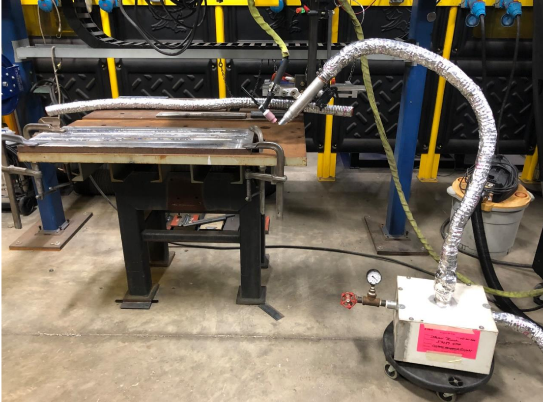
Figure 1. WeldVac System Component Overview
