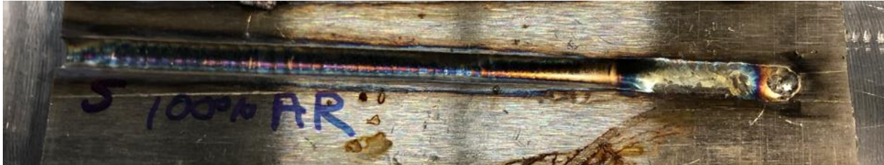
Figure 20. Second Gouge on 70-30 Cu-Ni
