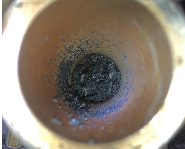
Figure 16. Typical Clogging in the One-piece Torch
