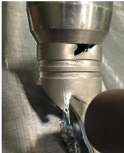
Figure 8. Melted tip with Significant Geometrical Changes to the Sip Port
