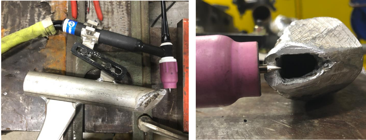
Figure 3. WeldVac Hand-Held Torch Version
