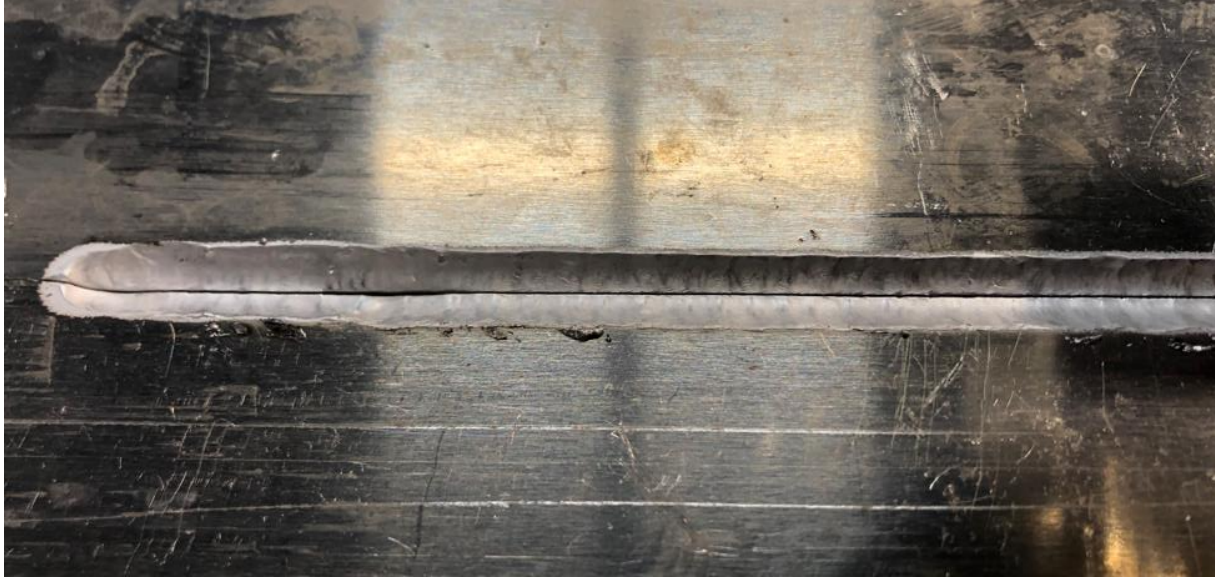
Figure 28. Back-Gouged Groove Trial on 5086 Aluminum Plate
