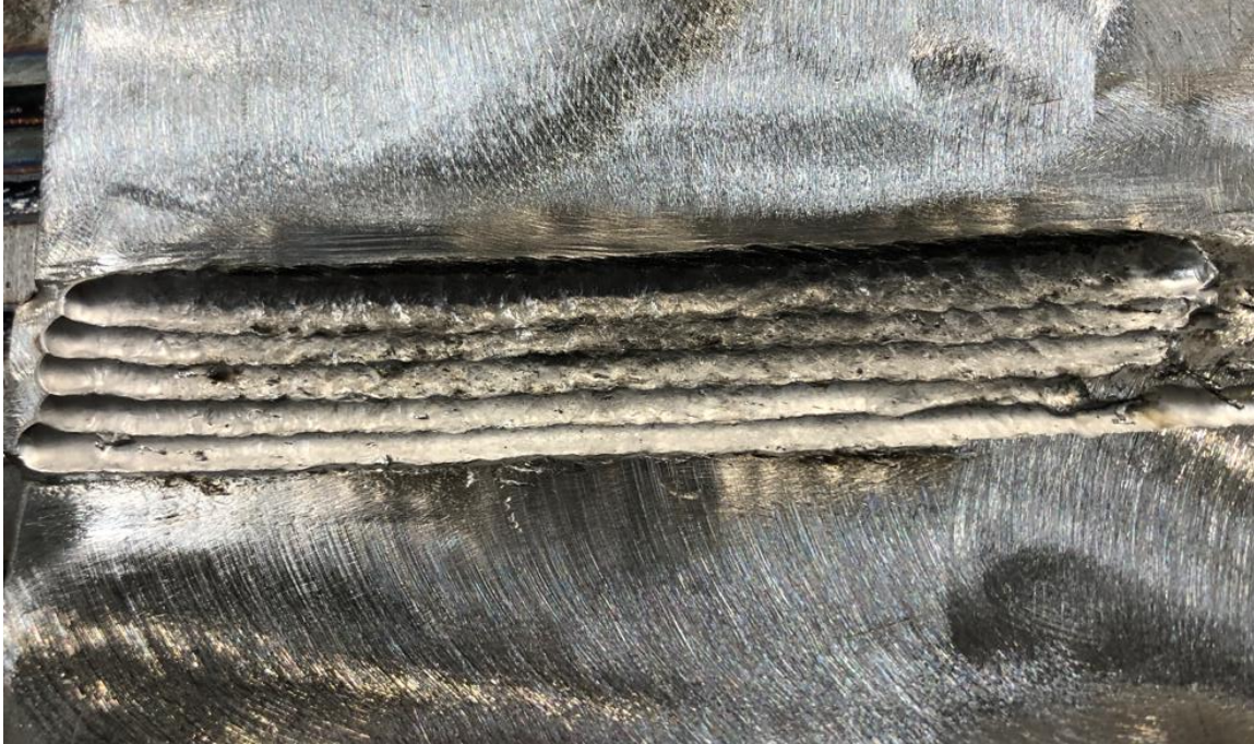
Figure 25. Complete Weld Reinforcement Removal from Aluminum Plate
