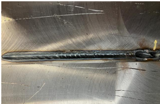
Figure 17. Single Gouge Pass on DH36 at Vigor Shipyard Demonstration
