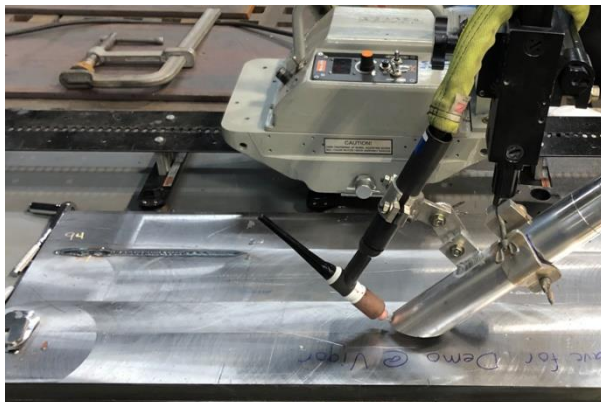
Figure 17. Single Gouge Pass on DH36 at Vigor Shipyard Demonstration
