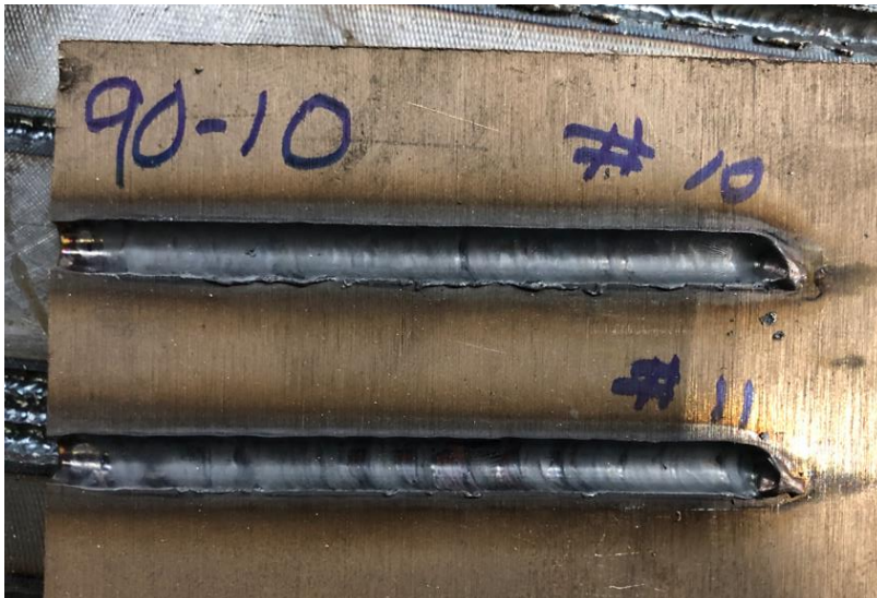
Figure 21. 90-10 Cu-Ni Gouges Using 75% Helium- 25% Argon Shielding Gas
