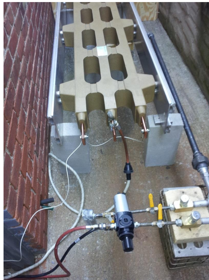
Figure 1: Set up showing 3 Phase IBP sample, Gas piping, and electrical connections.
