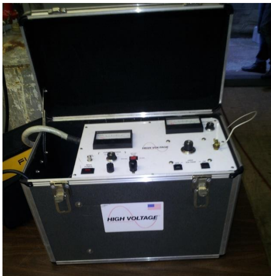
Figure 2: Hi-Pot used to provide 8 kV to sample
