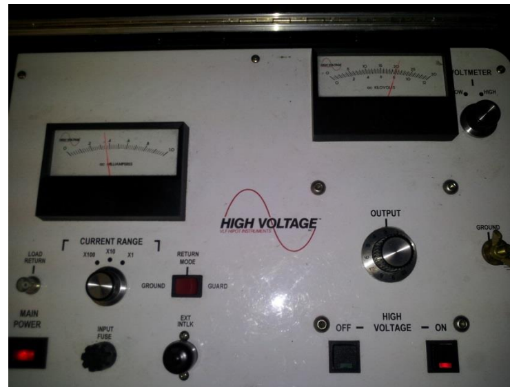
Figure 5: Hi-Pot set at 8 kV and leakage current holding steady at 3.6 mA
