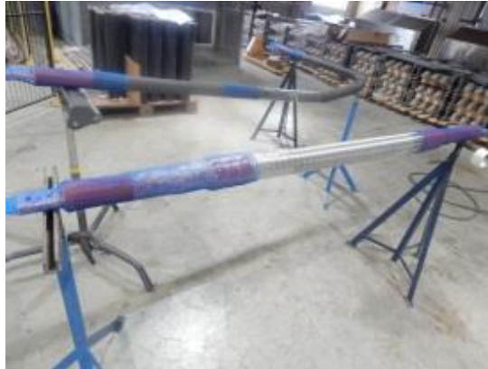
Figure 6: Telefen Single Phase IBP rated at 15 kV at 1300 Amps.
