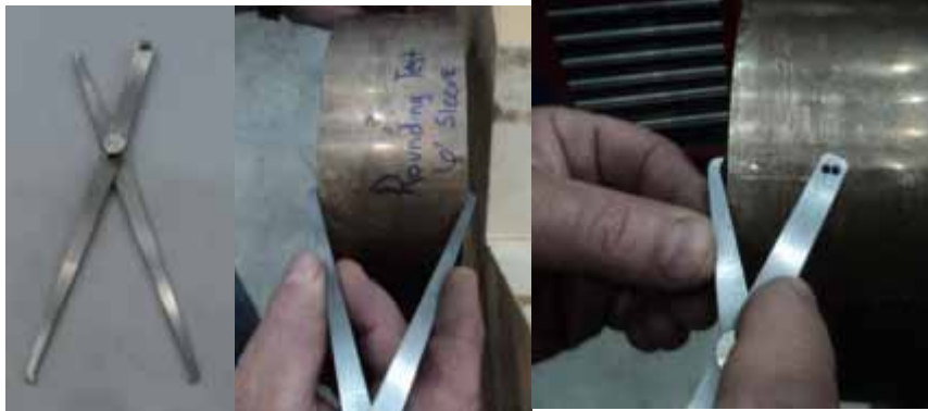
Divider Tool to Scribe Setback Points on Sleeve Fittings
