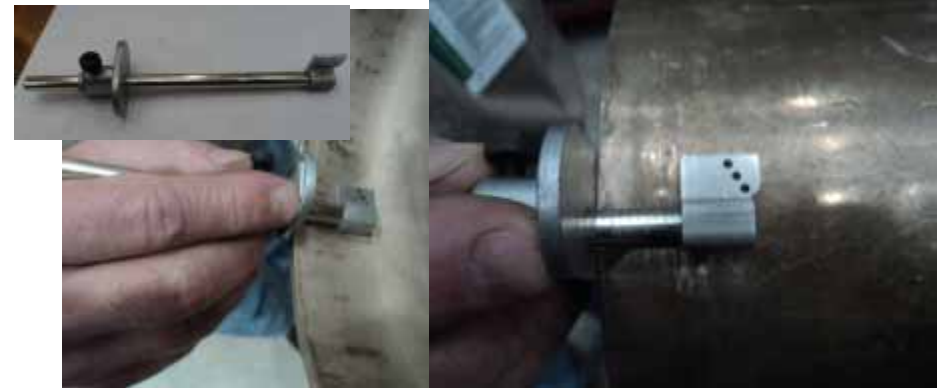
Depth Gauge Tool to Scribe Setback Points for Belled-end Fittings
