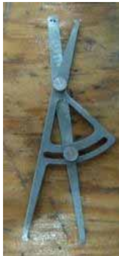
Divider Tool to Scribe Setback Points on Sleeve Fittings
